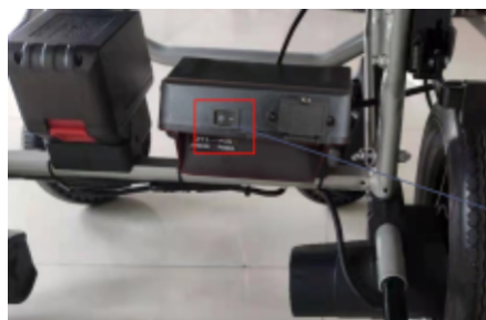
Main Power switch
