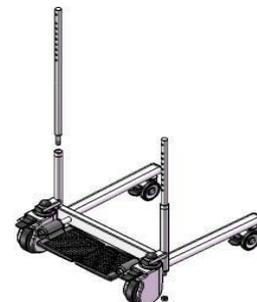
b) Place the handle part into the right shaft, as illustrated on the left :
