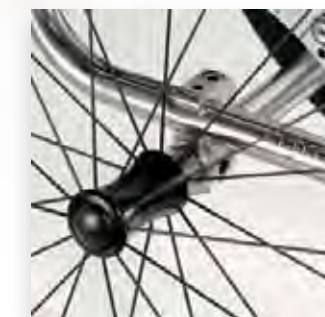
Asse regolabile. Adjustable centre of gravity axle.
